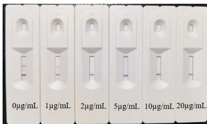
图 3.8 样品中不同浓度阿维拉霉素的检测结果 Fig. 3.8 Detection results of different concentrations of avilamycin in samples
